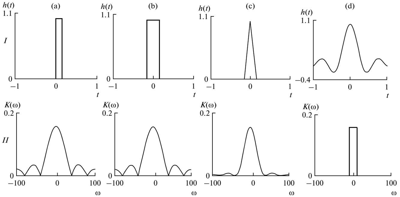
**Fig. 7.** (*I*) Impulse and (*II*) frequency characteristics of interpolating filters: (a) a zero-order nonsymmetric element, (b) a zero-order symmetric element, (c) a first-order element, and (d) a lowpass filter.
