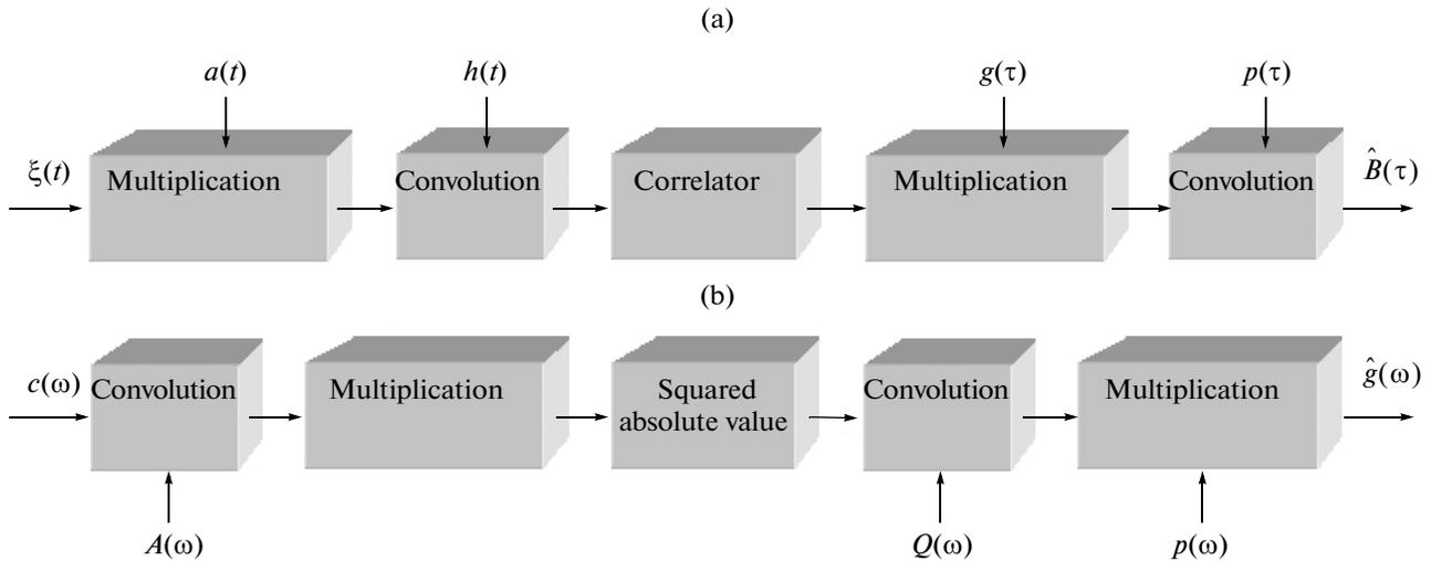
**Fig. 5.** Flowchart of introduction of the Kravchenko–Rvachev weighting and smoothing functions (windows) for estimating (a) correlation function  $\hat{B}(\tau)$  and (b) the spectrum.
