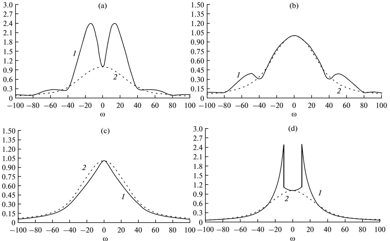
**Fig. 8.** Comparison of (curve *1*) the normalized spectra  $G_{\Delta}(\omega)/G_{\Delta}(0)$  of the process under study and (curve *2*) the optimal case  $G_{opt}(\omega)/G_{opt}(0)$  for zero-order (a) nonsymmetric and (b) symmetric elements, (c) a first-order element, and (d) a Kotelnikov ideal lowpass filter.
