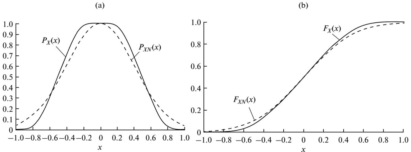
**Fig. 2.** Behavior of the (a) probability density and (b) distribution function: the (solid line) Kravchenko–Rvachev and (dashed line) Gaussian dependences.
