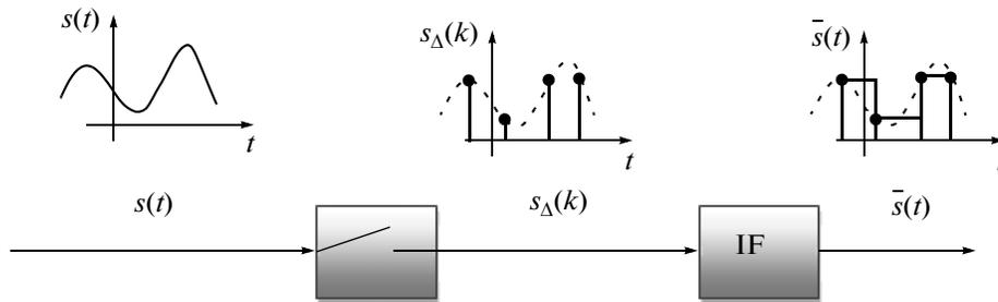
**Fig. 6.** Procedure of discretization and restoration of continuous signal  $s(t)$ .
