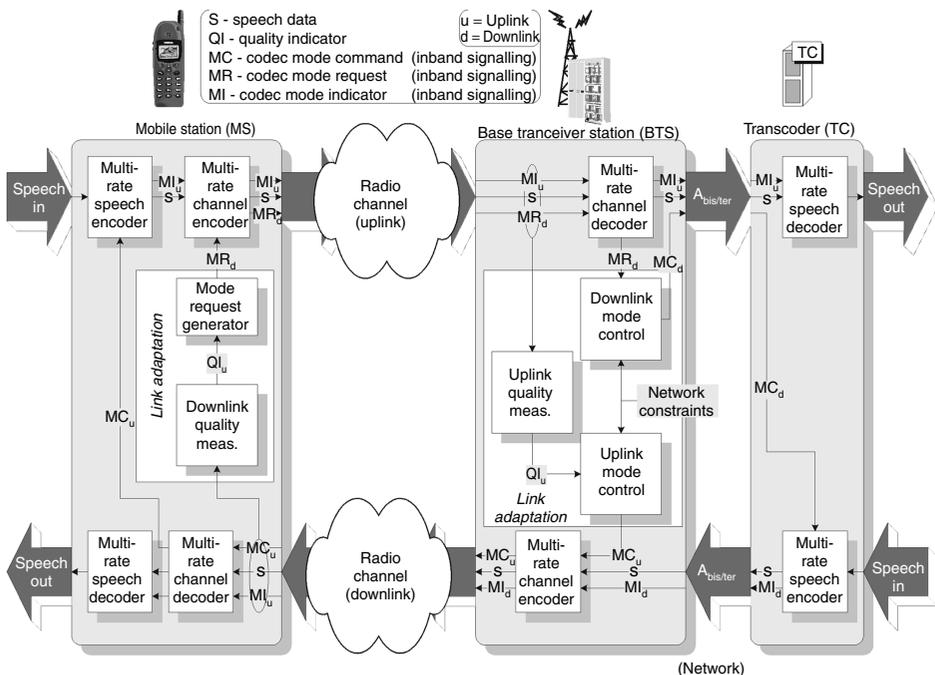
Figure 1.2. Block diagram of the AMR codec system
