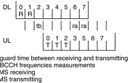
**Figure 1.22.** Extended dynamic UL allocation example
