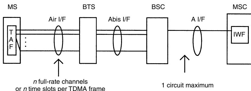
**Figure 1.3.** Network architecture for supporting HSCSD
