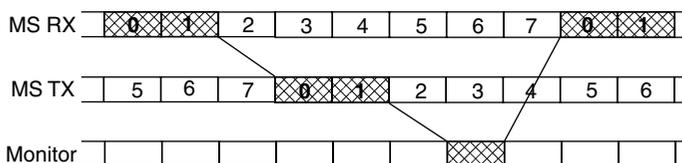
**Figure 1.4.** Double-slot operation in the air interface
