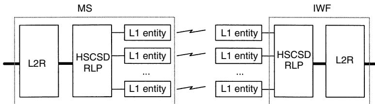
**Figure 1.5.** The HSCSD concept in non-transparent mode
