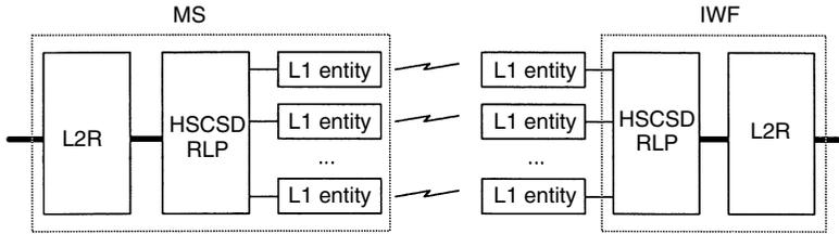
**Figure 1.5.** The HSCSD concept in non-transparent mode
