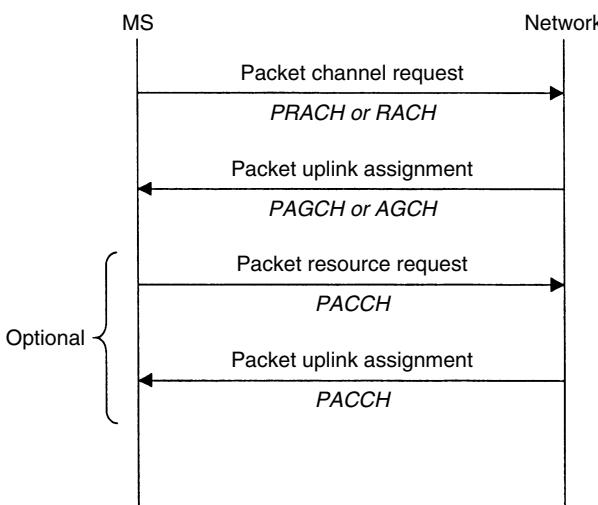
**Figure 1.23.** Access and allocation for the one or two-phase packet access, uplink packet transfer
