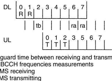
**Figure 1.22.** Extended dynamic UL allocation example
