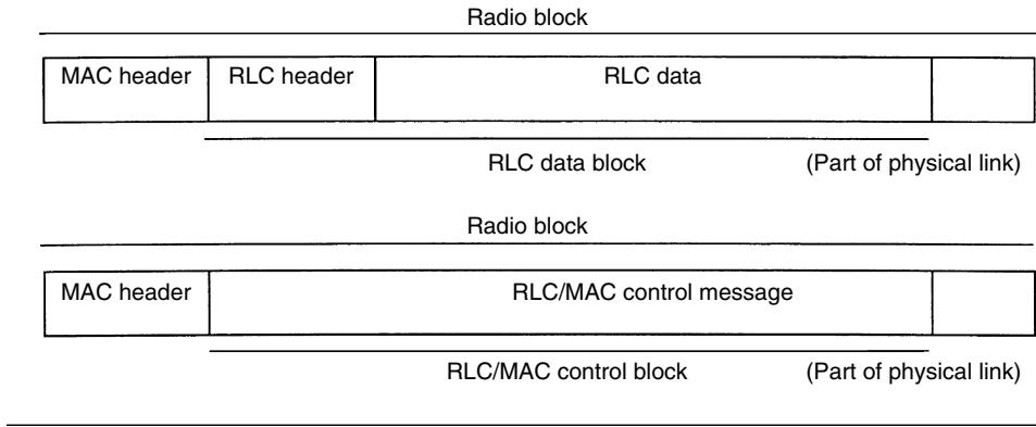
**Figure 1.17.** Radio block structures [14]
