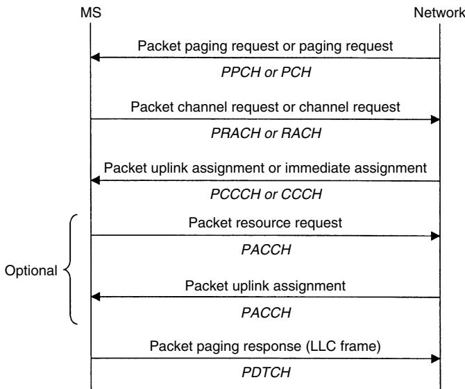
**Figure 1.24.** Paging message sequence for paging, downlink packet transfer
