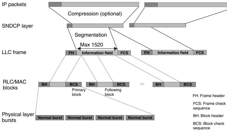
**Figure 1.20.** Transmission and reception data flow
