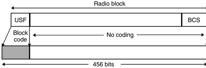
**Figure 1.19.** Radio block structure for CS-4 [14]
