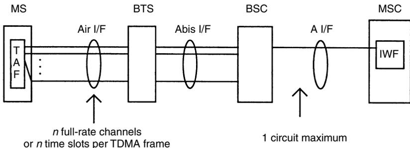
**Figure 1.3.** Network architecture for supporting HSCSD
