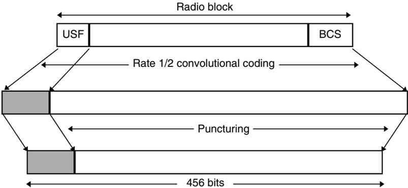
Figure 1.18. Radio block structure for CS-1 to CS-3
