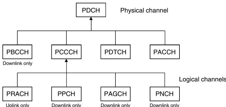
**Figure 1.15.** GPRS logical channels
